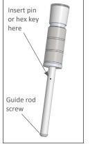
5. When you are satisfied with your spring selection, clean the guide rod threads and screw with solvent and dry completely. Install the guide rod screw with thread locker and tighten to 40-60 in-lbs. Some newer SCS kits come with screws pre-loaded with thread locker. The preloaded thread locker is only reusable two or three times. If you need to apply thread locker, we recommend a semi-permanent product such as Loctite® 243. If applying new thread locker, follow the accompanying instructions.
